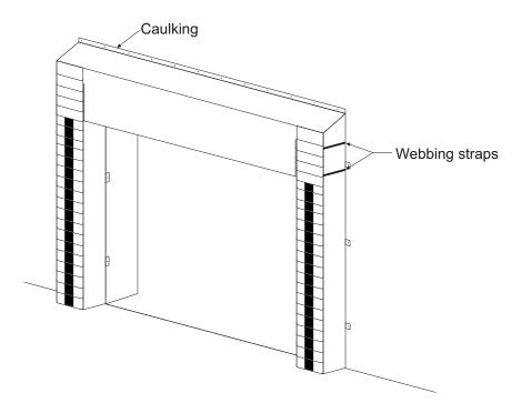
If the dock seal is incorrectly specified and/or misapplied for the application, not only will the seal be ineffective, but it may result in damage to the building and the loading dock seal. Adequate dock bumper projection is extremely important for the long life of the loading dock seal.
